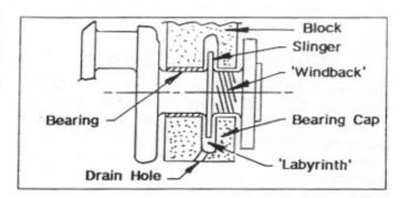
It works as follows, oil escaping rearward from the rear main bearing journal is thrown into the labyrinth by the rotating oil slinger on the crankshaft. The oil drains back into the sump via holes in the rear main bearing cap. Any excess oil that escapes rearward past the slinger is 'wound back' by the reverse thread machined into the crankshaft. You can see how excess crankcase air pressure can enter the labyrinth via the oil drain holes in the rear cap and blow oil out the back of the engine.
