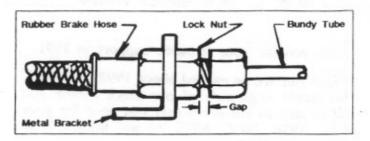
If there is no gap and the nuts are touching, the hydraulic joint may not be fully tight. Leaks lead to brake failures. You can reduce the thickness of the lock nut to solve the problem. Most installations had special thin nuts fitted in production.
